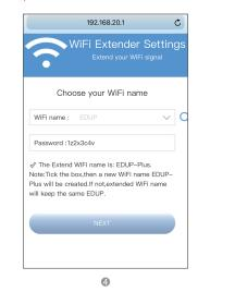
6. This interface displays the wireless settings status of the current device, then click to complete the settings.
